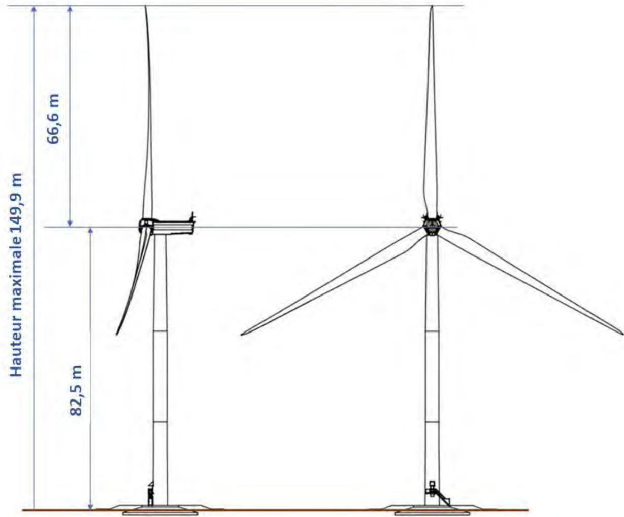
FIGURE 63 - CARACTERISTIQUES D'UNE EOLIENNE
